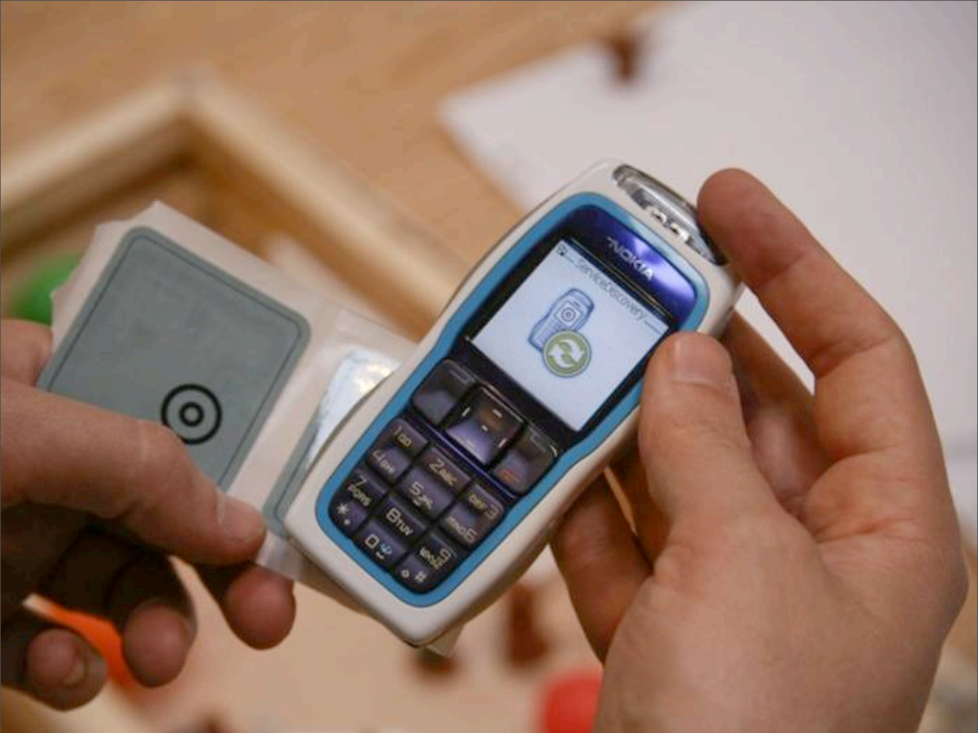
NFC extends RFID to provide a mechanism for two-way data transfer
