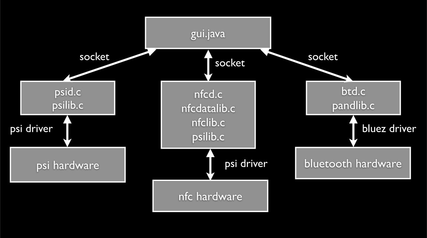
Once the hardware was in place, it took a lot of tweaks of firmware to get the phone to work. The gist of what was done was to prevent the phone from loading it's drivers and instead load the PSI kernel module.
