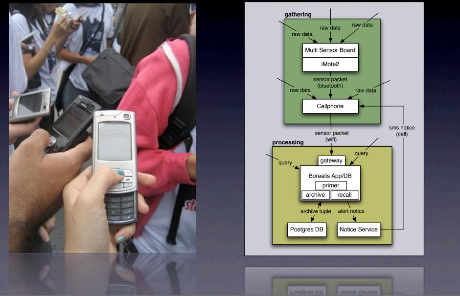
The SensorPlanet project builds an open global mobile device centric research platform for wireless sensor network research, akin to somewhat analogous platform for backbone network services called PlanetLabs.
