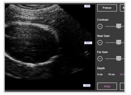
Mobile Midwives' Ultrasound is an inexpensive portable ultrasound device designed for midwives in low-income regions. The device helps identify three common obstetrical conditions: placenta previa, multiple gestations, and breech presentation.
