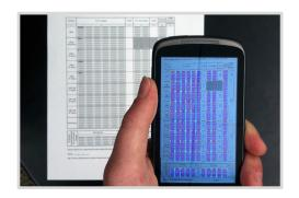
FreeForm is a mobile form scanning system that uses computer vision to automate the capture of data from paper forms. The system could significantly reduce the cost of digitizing data in a number of domains.
